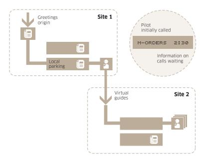
On a given local site, "Remote Groups" are assigned, which represent images of remote distributions. The remote distribution consists of a virtual pilot (dedicated), and a virtual queue, served by the groups of the remote node.
